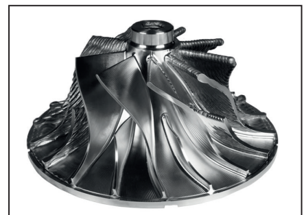
Partly machined part
